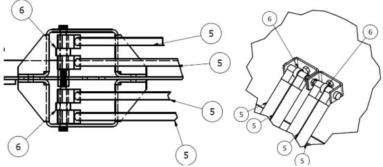
5 Gas Springs Per Cover (Left: Curb Connection, Right: Cover Connection)
