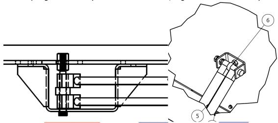
3 Gas Springs Per Cover (Left: Curb Connection, Right: Cover Connection)
