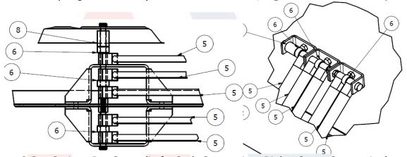
6 Gas Springs Per Cover (Left: Curb Connection, Right: Cover Connection)
